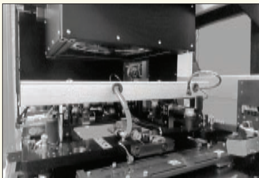
a customized UV-LED exposure system installed on a roll-to-roll machine
