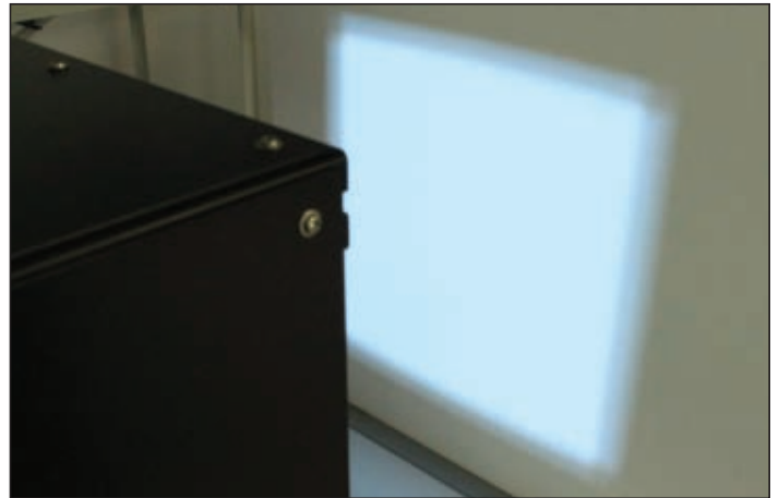
Highly homogeneous exposure area of 300x300 mm 2 is obtained with model UV-EXP300S.
