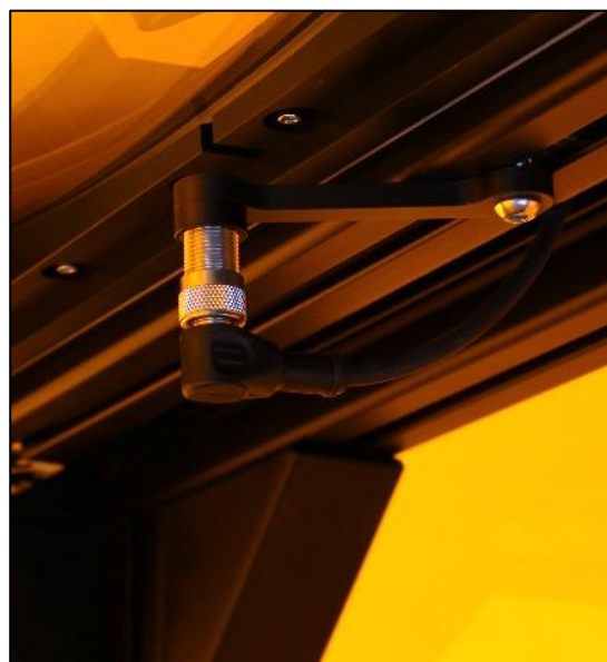
UV-SENS-GaP sensor installed on our UV-EXP system
