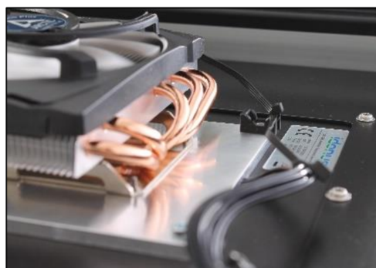
Detail of an air-cooled heat pipe system
