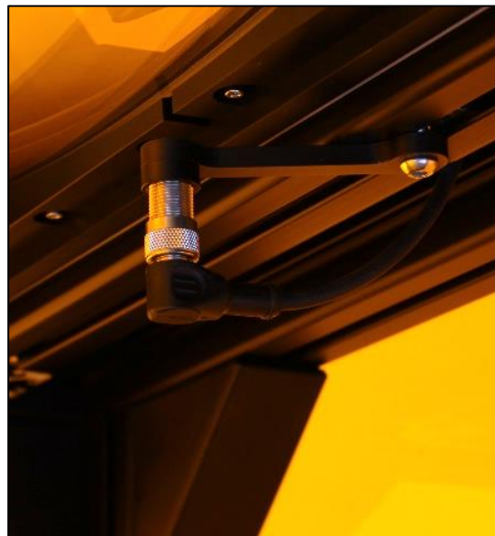
UV-SENS-GaP sensor installed on our UV-EXP system
