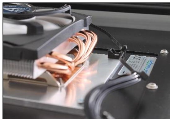
Detail of an air-cooled heat pipe system
