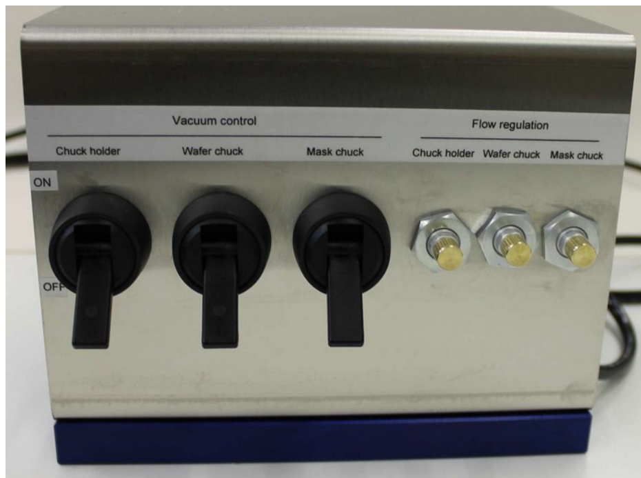
Pneumatic board for individual regulation of wafer, mask and chuck clamping during alignment.
