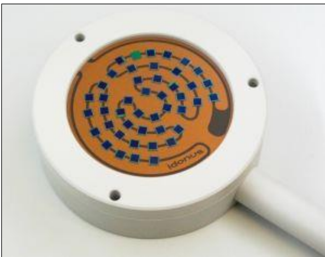
Figure 5: Electrostatic chuck with multiple chips.
